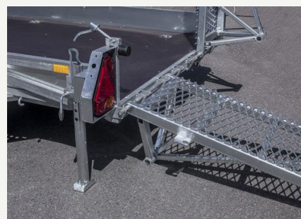
03 DRIVE-ON RAMP · DETAIL
