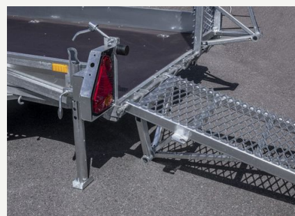
03 DRIVE-ON RAMP • DETAIL
